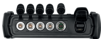
PPC-PAD-light for up to 4 analogue STAUFF Sensors with automatic sensor recognition and up to 2 analogue external sensors (e.g. 4-20 mA or 0-10 V).
