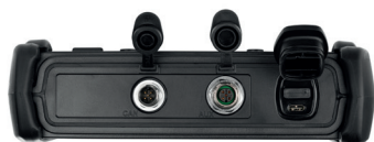
PPC-PAD-light-CAN-AUX for up to 6 STAUFF CAN Sensors (max. 50 m / 164 ft cable length) with automatic sensor recognition and up to 2 external analogue sensors (e.g. 4-20 mA or 0-10 V).
