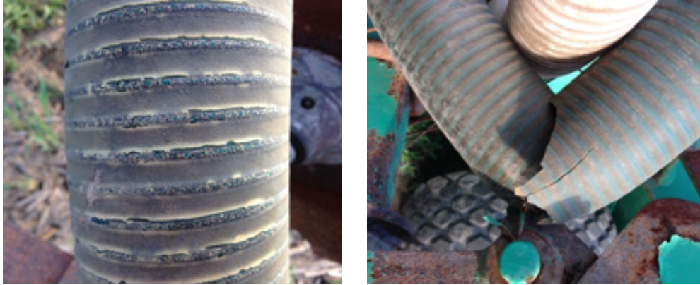
PVC Hose cracking due to UV exposure
